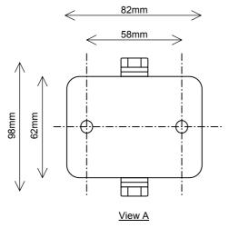
2off - Fixing holes 6.25mm (0.25") Dia.
